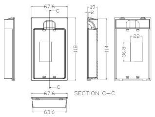
Fig.2-12 Little keyboard installed base dimension
