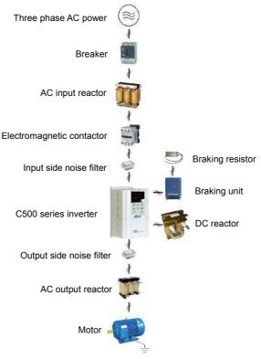
Fig.3-5 Connect the inverter to peripheral devices
