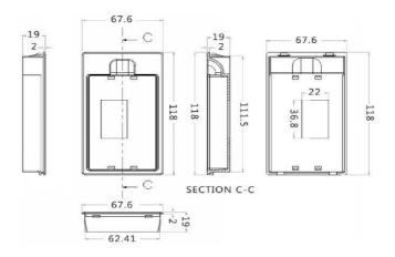
Fig.2-5 C10 Keyboard installed base dimension
