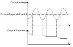
Fig.6-28 Over-voltage stall function
