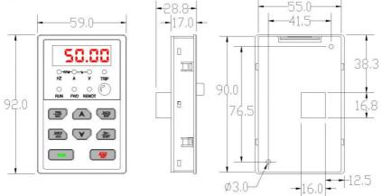
Fig.2-4 C10 Keyboard dimension C10 series(0.75-4KW) (mm)
