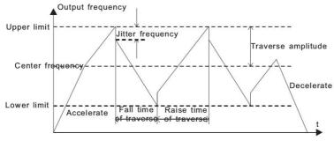
Fig.6-17 Traverse operation diagram
