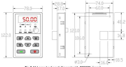
Fig.2-11 Large keyboard dimension(4~800KW) (mm)
