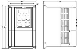
Fig.2-8 Standard dimension for C500 series inverter( 0.75KW~110KW)
