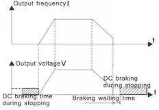
Fig.6-3 DC braking diagram
