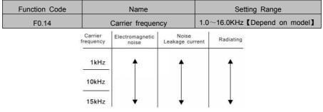
Fig.6-2 Effect of carrier frequency
