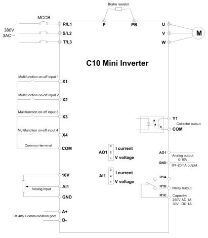
Fig.3-6 Standard wiring diagram
