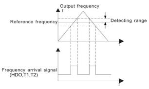
Fig.6-19 Frequency arriving detection diagram
