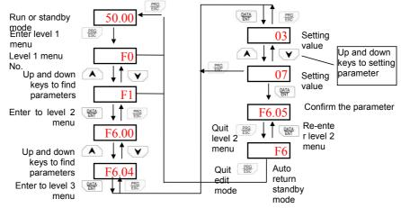
Fig.4-3 Function code parameter setting process
