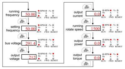
Fig.4-2 Under running condition, monitor parameters switching
