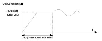
Fig.6-24 PID preset output diagram
