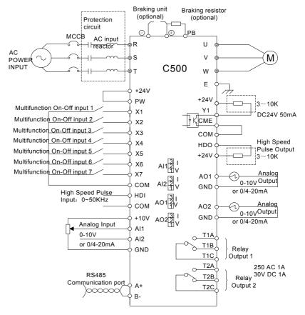
Fig.3-7 Standard wiring diagram
