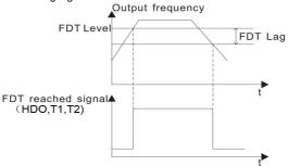
Fig.6-18 FDT level and lag diagram
