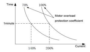
Fig.6-27 Motor overload protection coefficient
