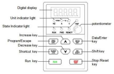
Fig.4-1 keyboard schematic diagram
