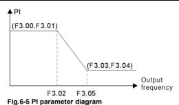
By setting the speed regulator's the proportion gain and the integral time Can adjust the ASR of the vector control dynamic response.if the proportion gain is increased or the integral time is decreased, The system dynamic response will be faster. However, if the proportion gain i s too large, the system tends to oscillate. If the integral time is too small, the system tends to o scillate And there may be speed difference. Please adjust these parameter according to actual situation.
