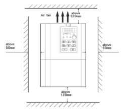
Fig.3-1 Spacing distance for installation
