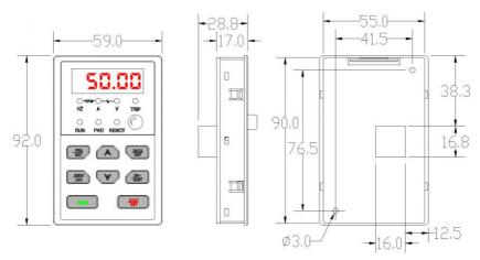
Fig.2-10 Little keyboard dimension(0.7~2.2KW) (mm)
