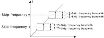
Fig.6-16 skip frequency diagram
