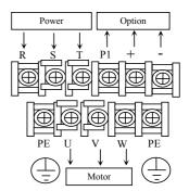
75~315KW main circuit terminals array
