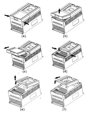
Fig.3-4 C500-4.0/5.5KW cover plate dismantlement and installation
